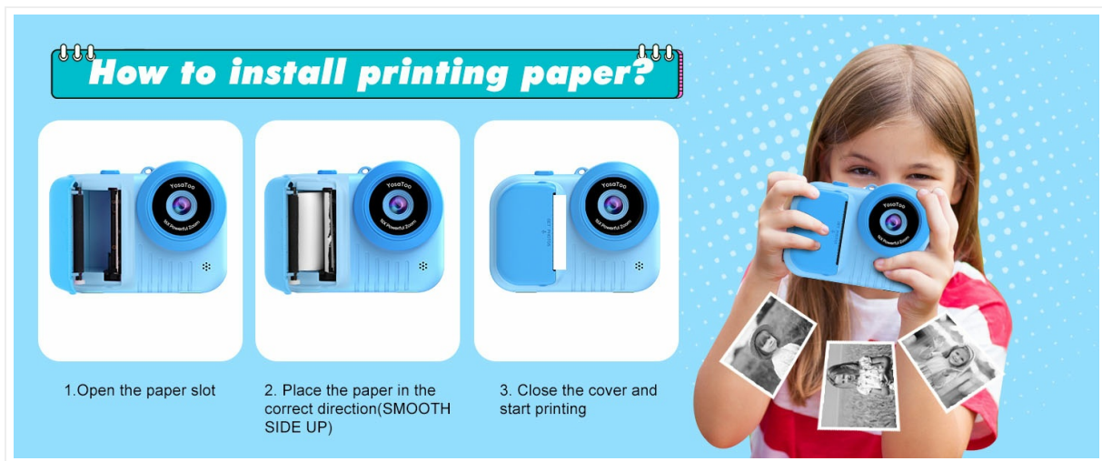
Image 3.2: Visual instructions for loading print paper: 1. Open the paper slot. 2. Place paper with the smooth side up. 3. Close the cover.
