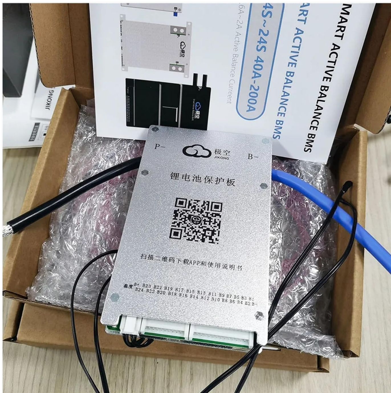
The Aoleaby JK Smart BMS BD6A24S6P unit, packaged with its instruction manual, ready for installation.
