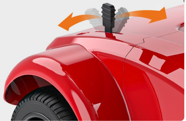
Figure 3: The switchable handbrake, which also controls power.
