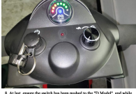
8. At last, ensure the switch has been pushed to the "D Model", and while you hold the key, you hear a "beep-beep", and the battery power display lighting on, that is mean you make it.
