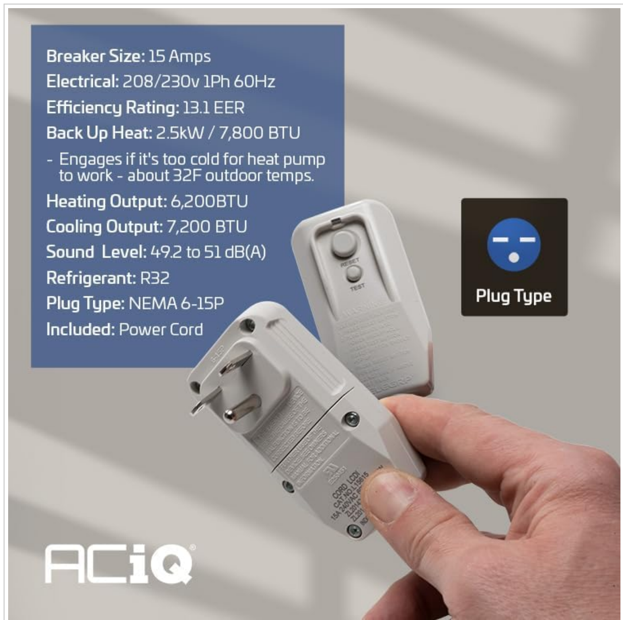
Image 4.2: A close-up of the NEMA 6-15P plug, alongside a summary of the unit's electrical and performance specifications.
