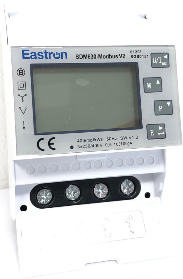
Figure 2: Front view of the meter with the terminal cover open, providing access to the main power and communication wiring terminals.
