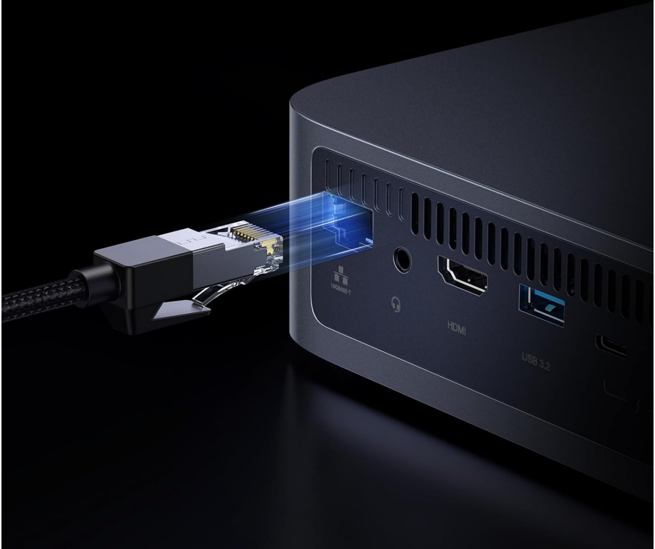
Figure 3.3: Network Connection via 10GbE Port
