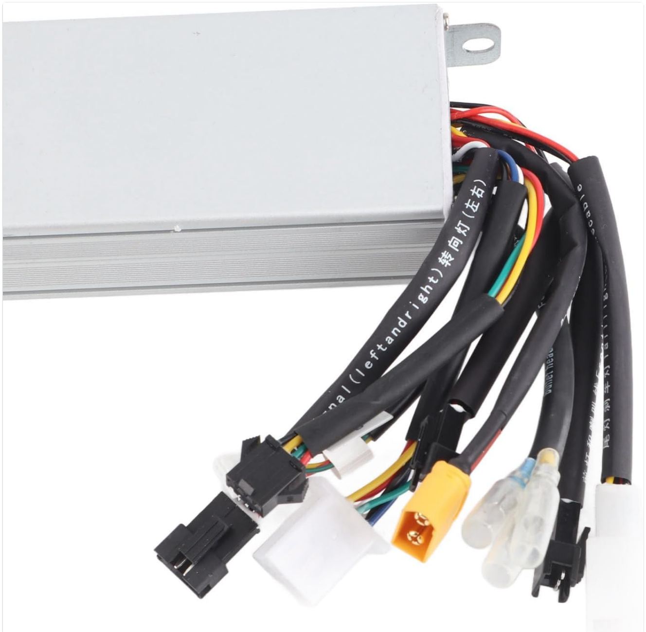
Figure 4.1: Detailed view of the controller's wiring harness.
