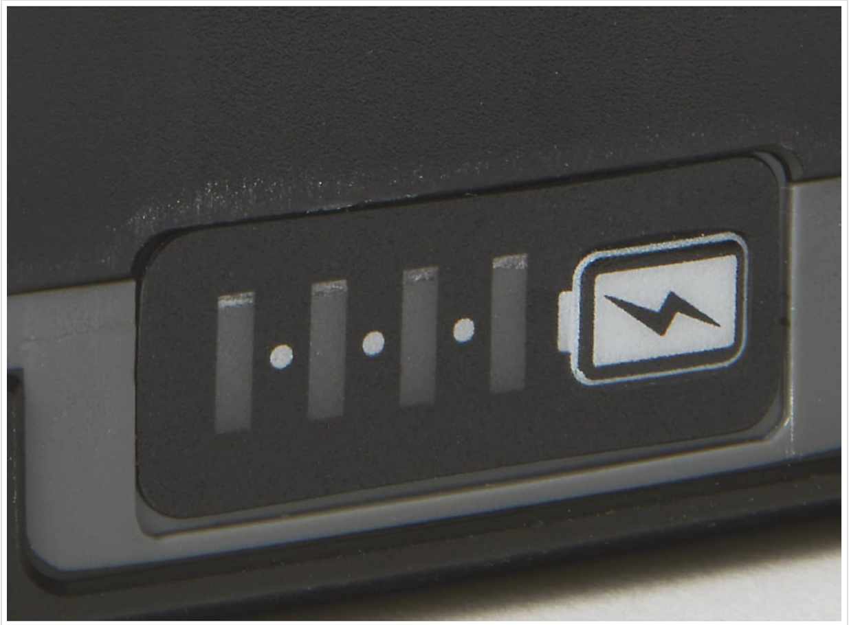
Image: A close-up view of the battery's fuel gauge, showing four illuminated bars, indicating a full or near-full charge.
