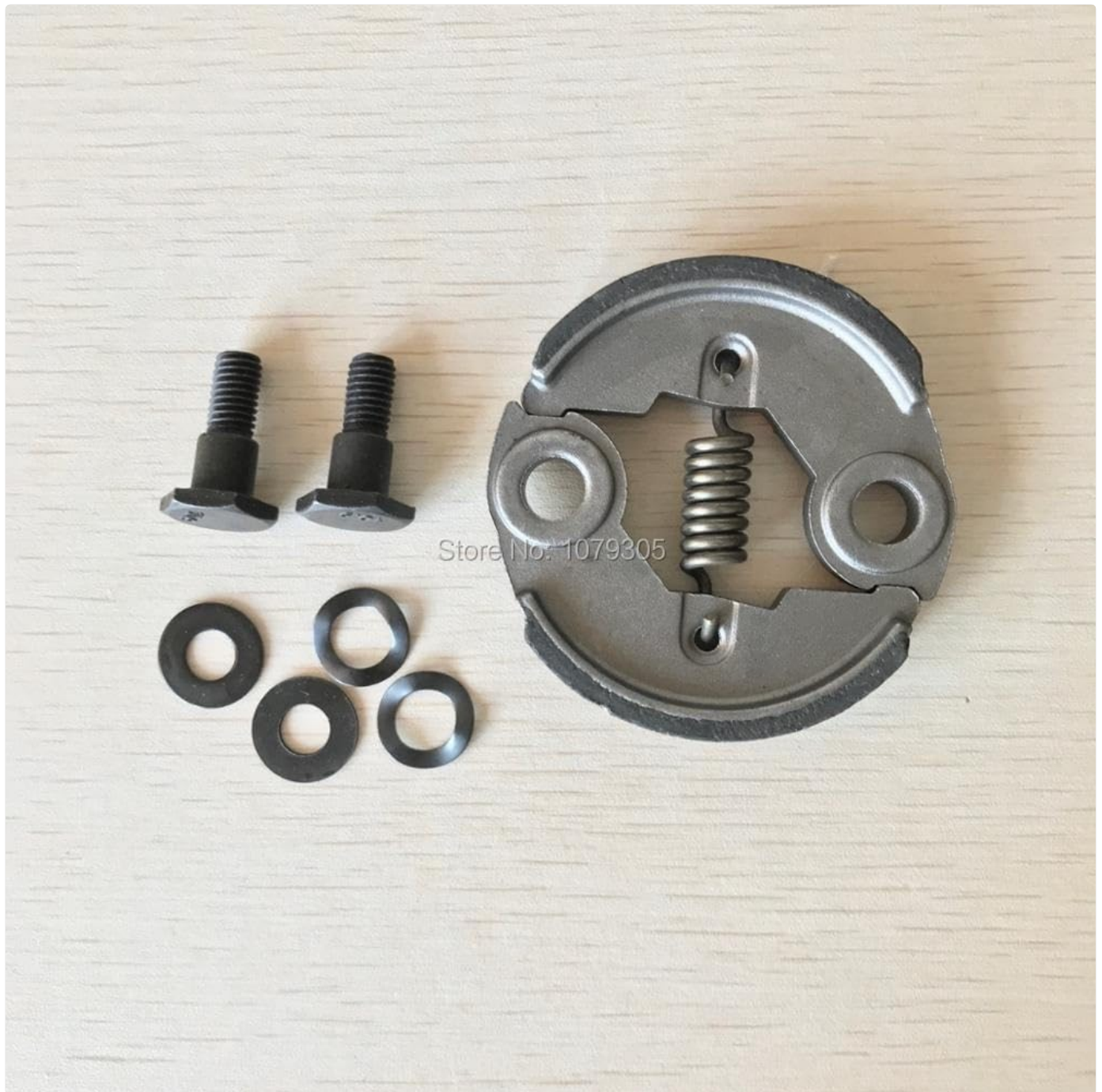
Figure 1: Complete Gerrit CG430 clutch assembly, including the main clutch unit, two mounting screws, and various washers.
