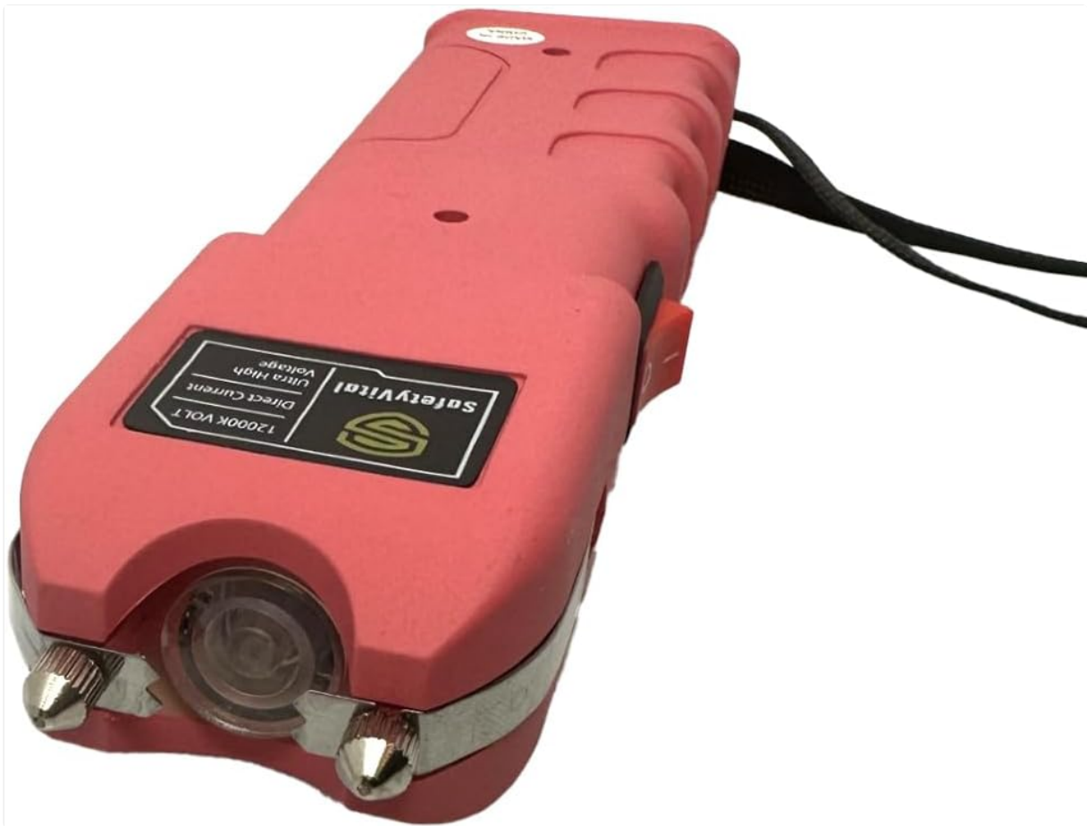
Figure 2: Front view of the stun gun, highlighting the stun electrodes and LED flashlight.
