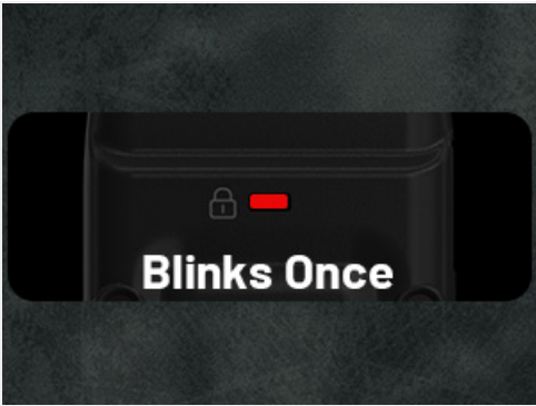
Figure 6: The red lockout indicator blinking once, confirming lockout mode engagement.
