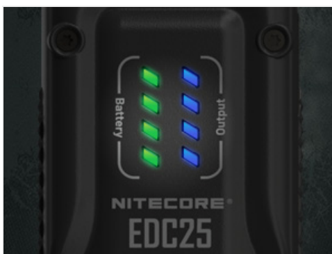
Figure 4: Battery (green) and Output (blue) indicator LEDs on the Nitecore EDC25.
