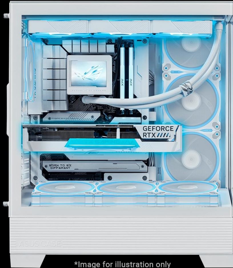
Figure 4: An internal view of the ASUS A31 Plus case, highlighting its spacious interior designed to support large graphics cards and 360mm radiators, indicating broad component compatibility.
