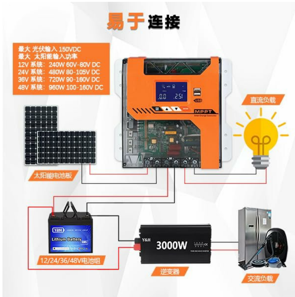
Image 4.1: Connection diagram showing solar panels, the MPPT controller, battery, inverter, and AC/DC loads. This illustrates the proper wiring sequence for a complete solar power system.
