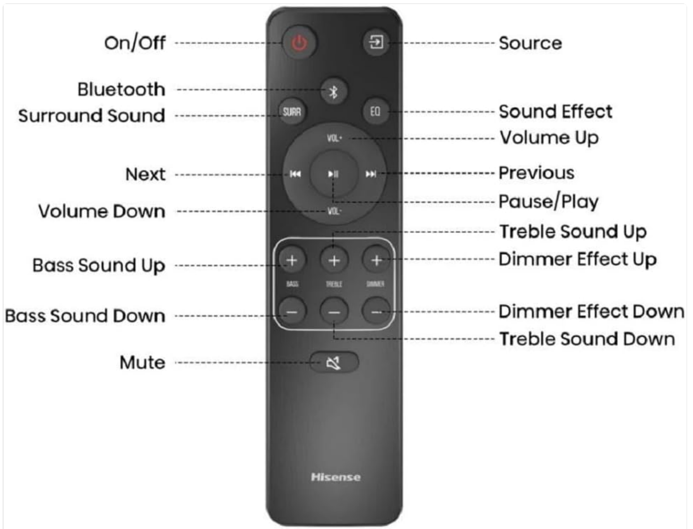
Image: Detailed layout of the Hisense AX5120G soundbar remote control, showing all buttons and their corresponding functions.
