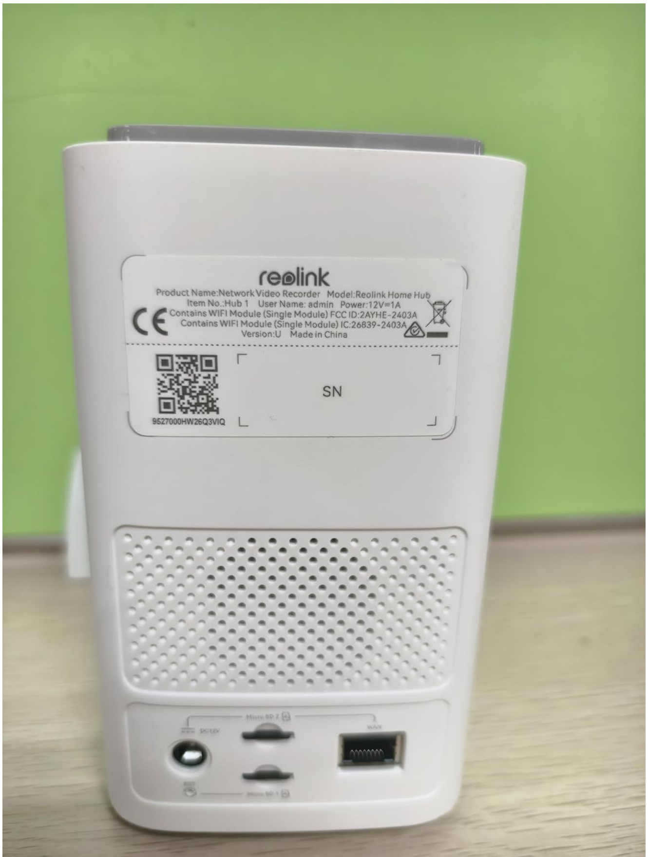
Image 3.2: The rear panel of the Reolink Home Hub, displaying the Ethernet port, power input, and microSD card slots.
