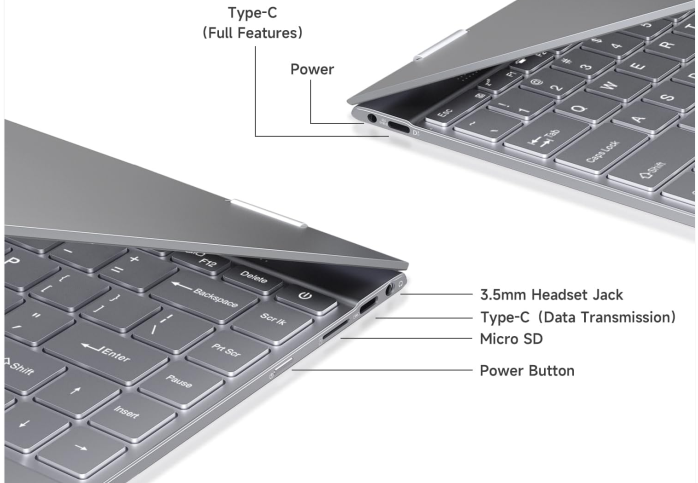
Figure 3.7: Detailed view of the laptop's ports, including two Type-C ports (one full-featured, one for data transmission), a 3.5mm headset jack, a Micro SD slot, and the power button.
