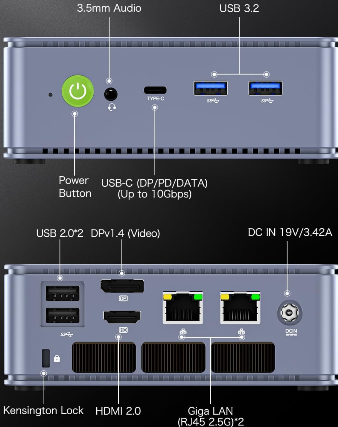
Figure 3.2: Front and rear panel interfaces of the GMKtec M5 Plus Mini-PC.
