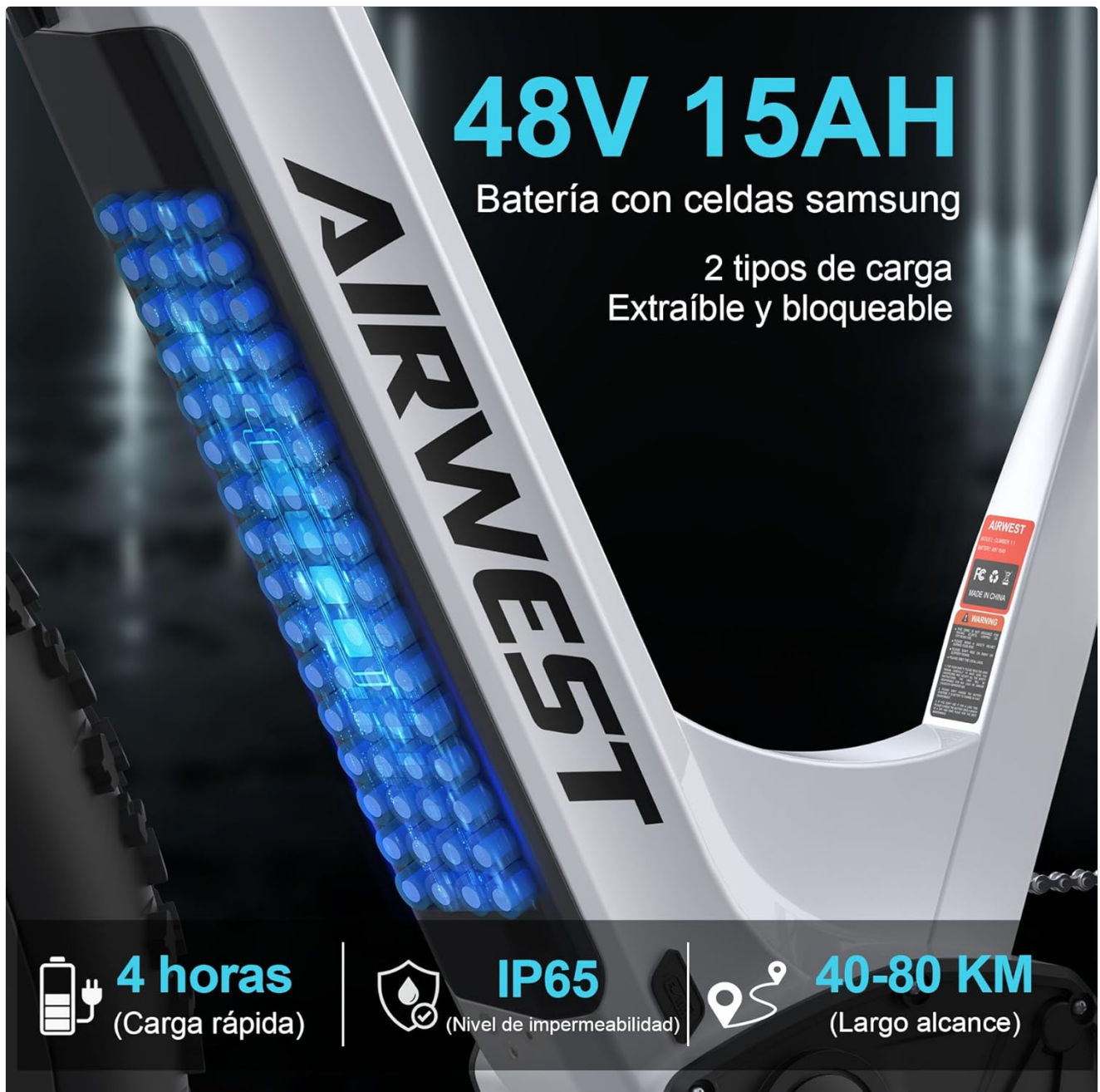
Figure 3.6: The 48V 15Ah Samsung battery, which can be charged on or off the bike. It features IP65 waterproofing and anti-theft locking.
