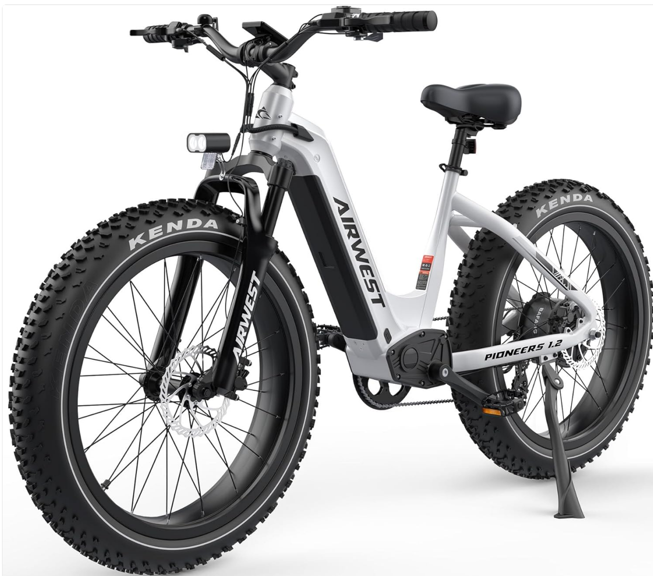
Figure 4.6: The airwest electric bicycle featuring its robust design, fat tires, and front suspension.
