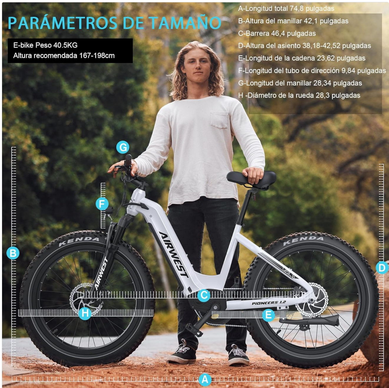
Figure 7.1: Detailed size parameters of the airwest electric bicycle.
