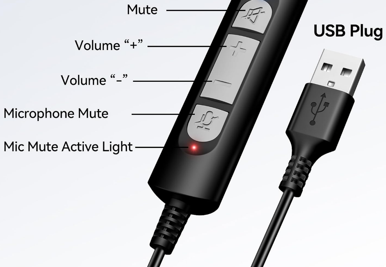
Image 5.1: Detailed view of the in-line control unit.
