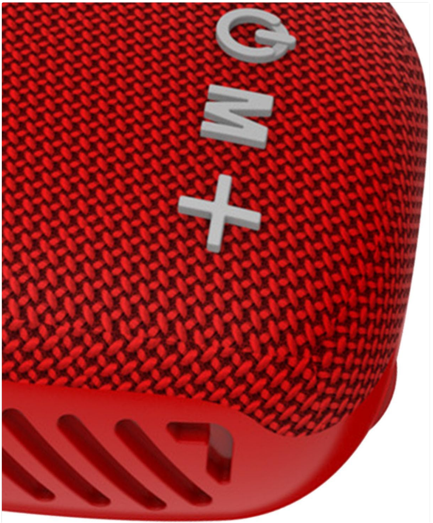
Figure 4.2: Close-up of the speaker's control panel, featuring the volume up (+), mode (M), and volume down (-) buttons.
