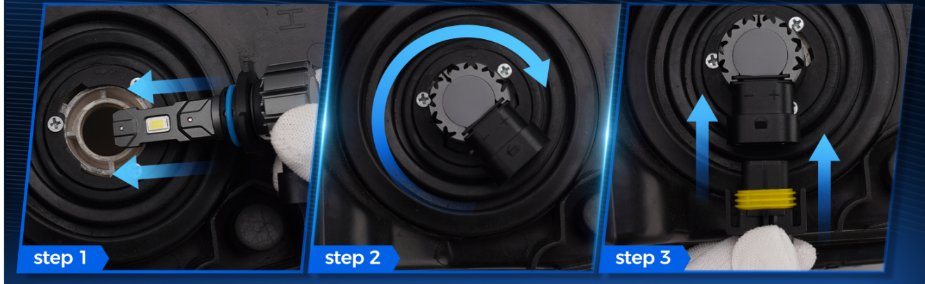
Image 4.2: A three-step visual guide illustrating the simple plug-and-play installation process for Marsauto M1S LED bulbs, from insertion to connection.
