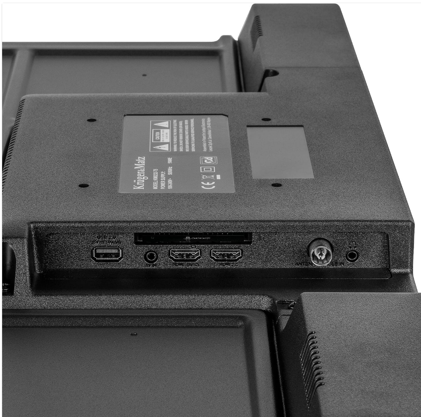
Figure 4.2: Rear connectivity ports.
