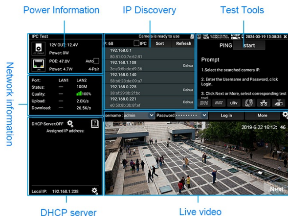
Image 6.3.2: The IP Discovery function scanning for devices and the ONVIF interface showing live camera feed and login status.
