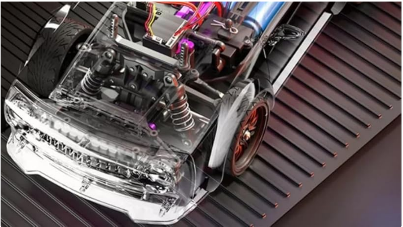
Image: Transparent view of the chassis, illustrating the internal body structure, motor, and cooling system. This design aims to protect the motor.
