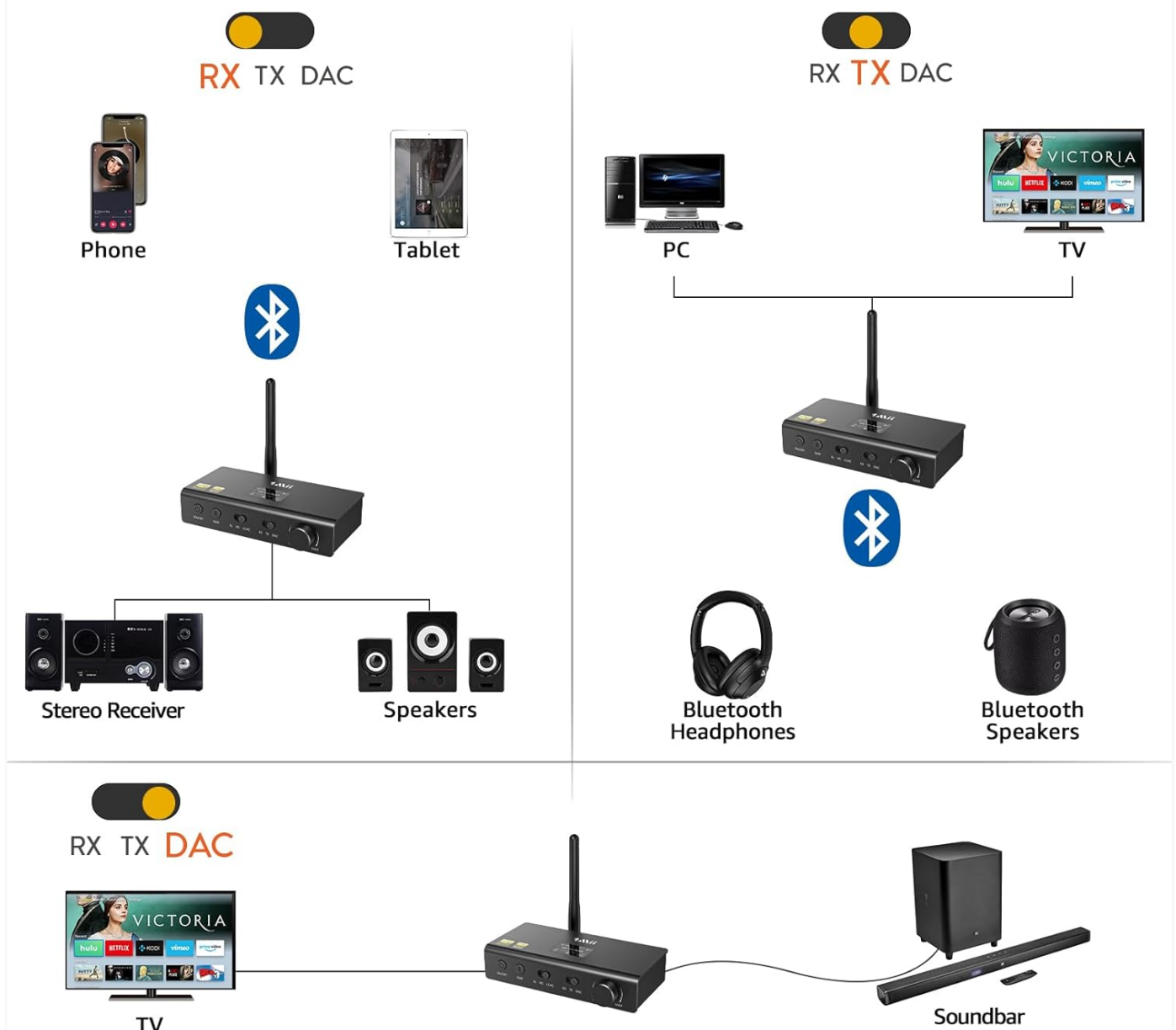
Image: An overview diagram illustrating the 3-in-1 functionality of the 1Mii DS700, showing its use as a receiver (RX), transmitter (TX), and DAC with various audio devices.
