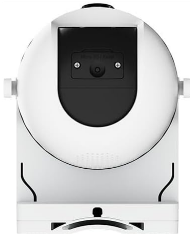
Figure 3.4: Bottom View - Reveals the MicroSD card slot, protected by a cover, for local storage of recordings.
