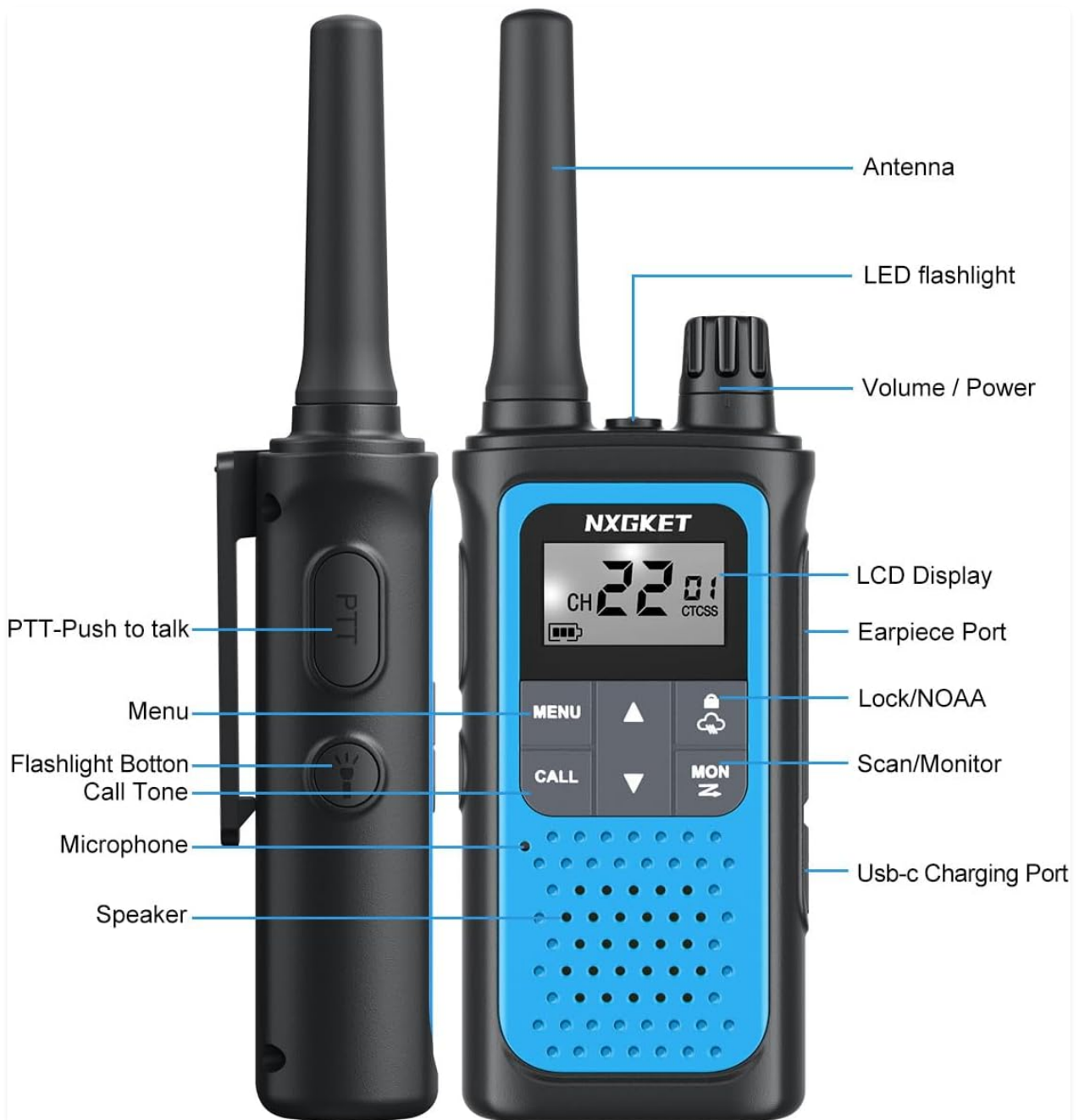
Figure 3.1: Key Components and Controls of the Walkie Talkie.
