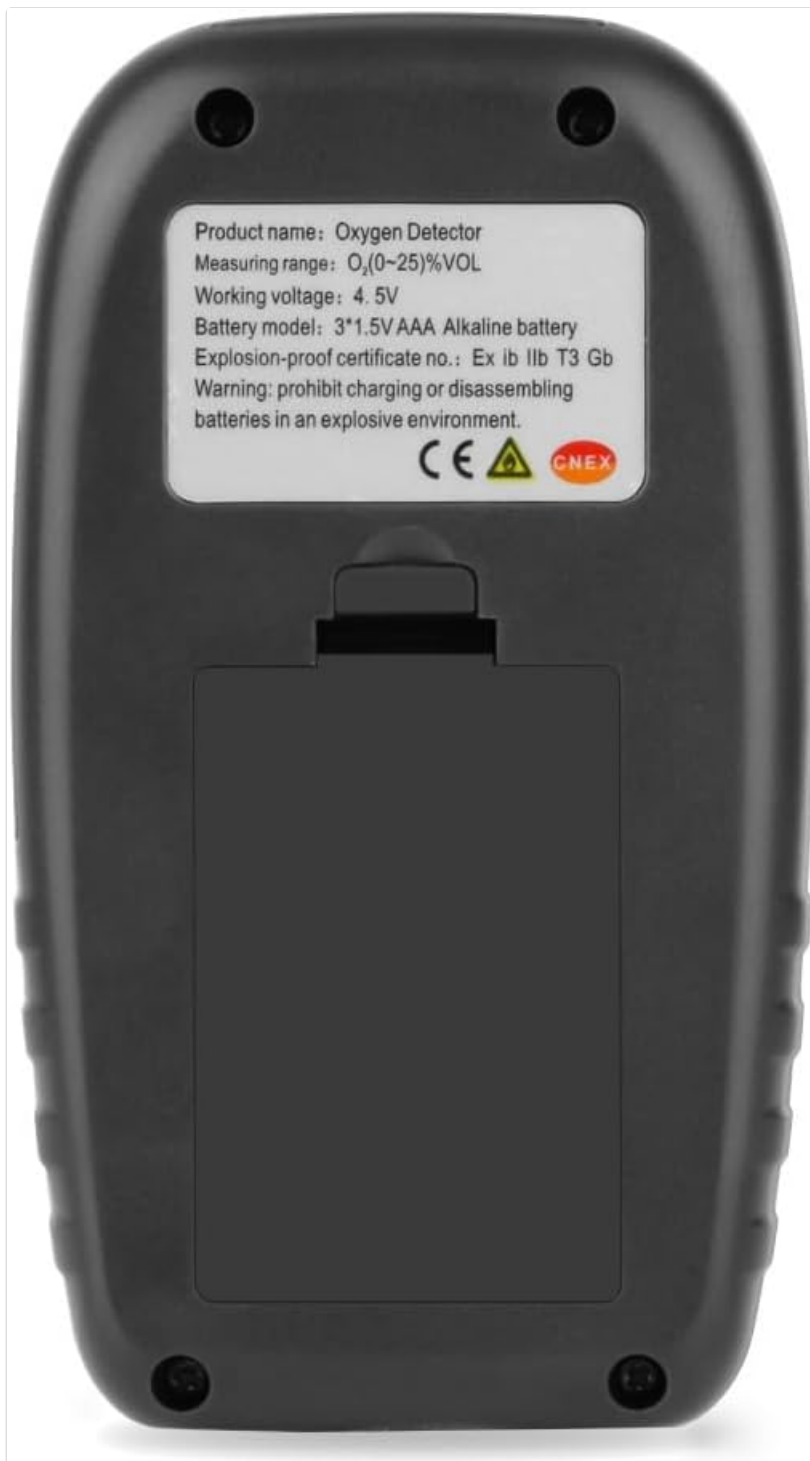
Figure 7: Back view of the DEWIN WT8821 Oxygen Detector, displaying the product label with key specifications and the battery compartment.
