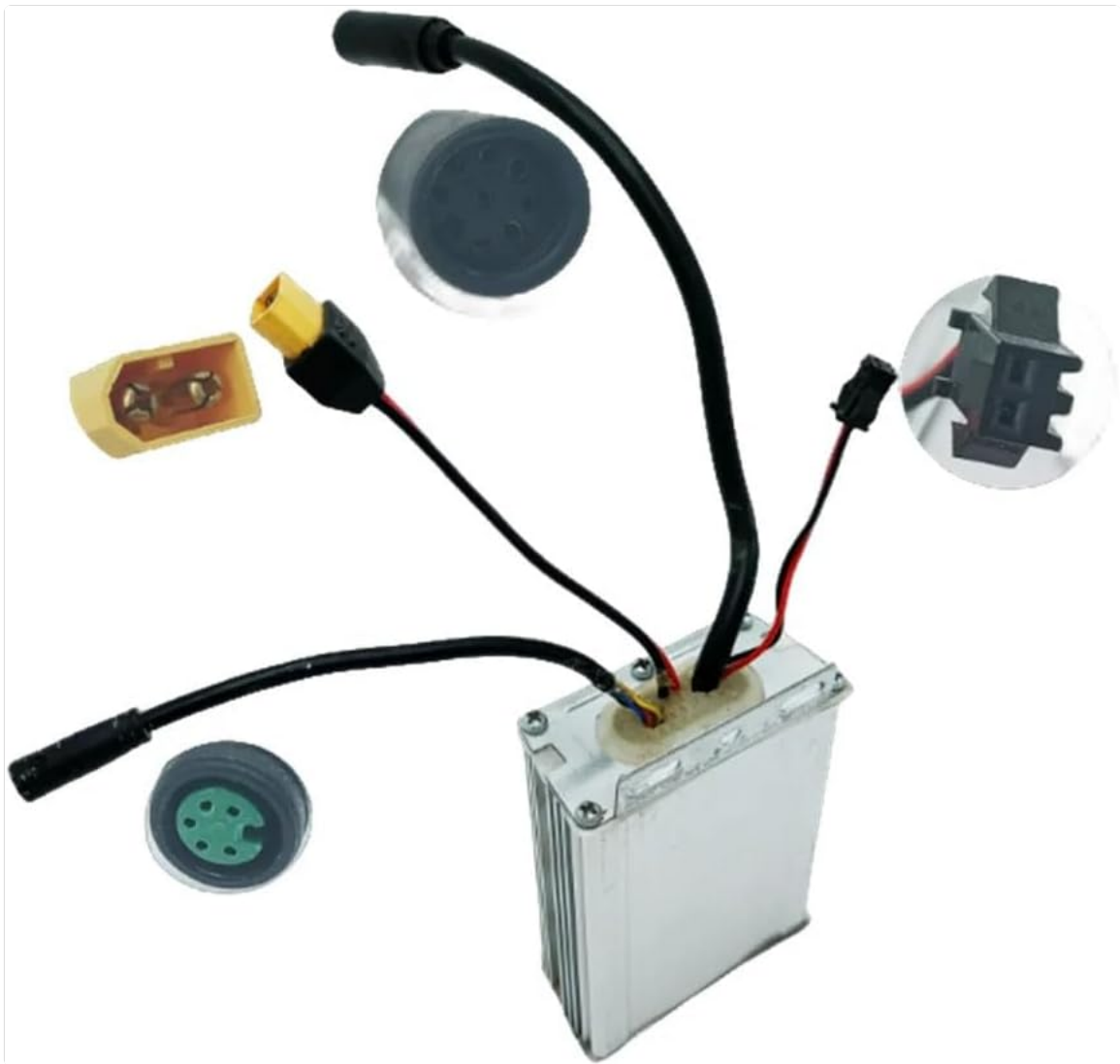
Image 3: The XIBANY controller displaying multiple types of connectors, including a multi-pin circular connector, a yellow XT60-style connector, and a rectangular 3-pin connector, illustrating the variety of connections required.
