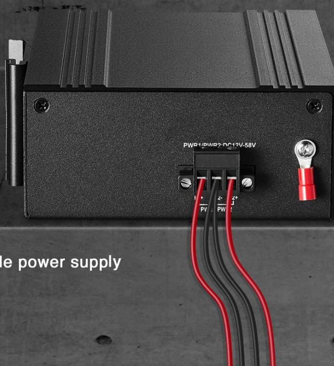
Figure 3: Dual redundant power inputs (PWR1, PWR2) supporting DC12-58V, with features like wide voltage input, redundancy power supply, 4.0A overcurrent protection, and reverse connection protection. Note: Power supply is not included.
