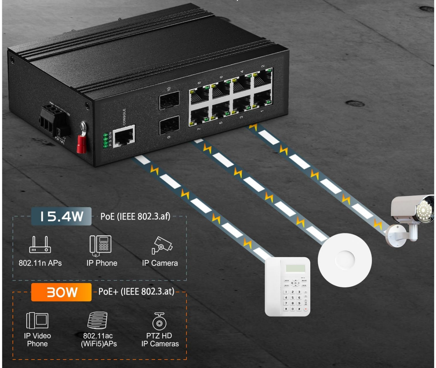
Figure 4: Smart PoE+ support compliant with IEEE 802.3af/at PoE standards. Illustrates 15.4W PoE (IEEE 802.3af) for devices like 802.11n APs, IP Phones, and IP Cameras, and 30W PoE+ (IEEE 802.3at) for IP Video Phones, 802.11ac (WiFi5) APs, and PTZ HD IP Cameras.
