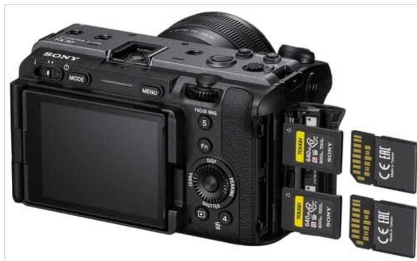
Image: Rear view of the Sony FX30 showing the open memory card slots with two SD cards partially inserted.
