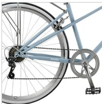
Image: Close-up of the Shimano 7-speed rear derailleur and cassette. This component manages the chain movement across the gears for speed changes.
