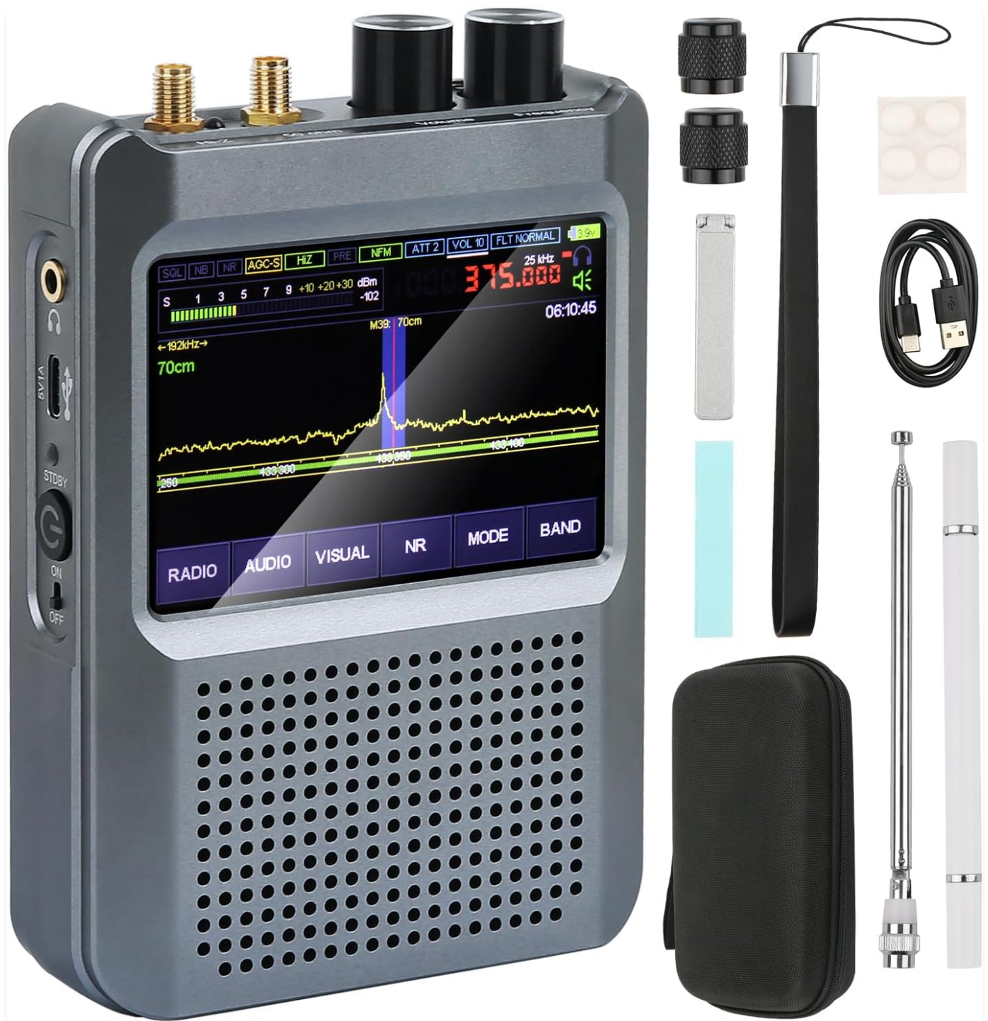
Figure 1: Malachite DSP2 SDR Radio Receiver and included accessories.
