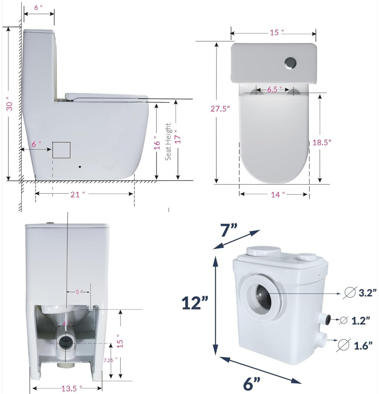
Image: Detailed product dimension diagrams for both the toilet unit and the macerator pump.
