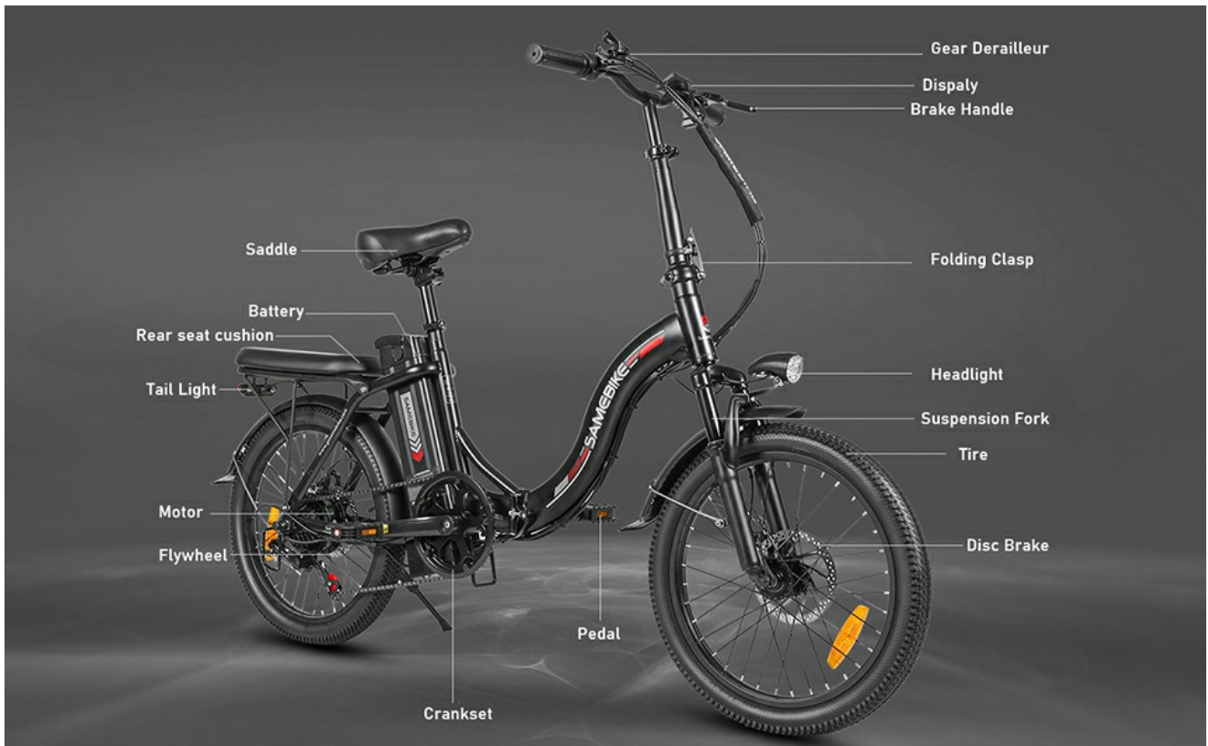
Figure 3.1: Overview of the SAMEBIKE CY20 Electric Bicycle with key components labeled, including the headlight, suspension fork, disc brake, pedal, crankset, motor, flywheel, tail light, rear seat cushion, battery, saddle, folding clasp, display, and brake handle.
