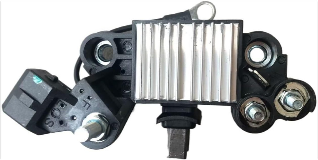
Figure 4: Back view of the voltage regulator brush set, showing the heat sink for thermal management.
