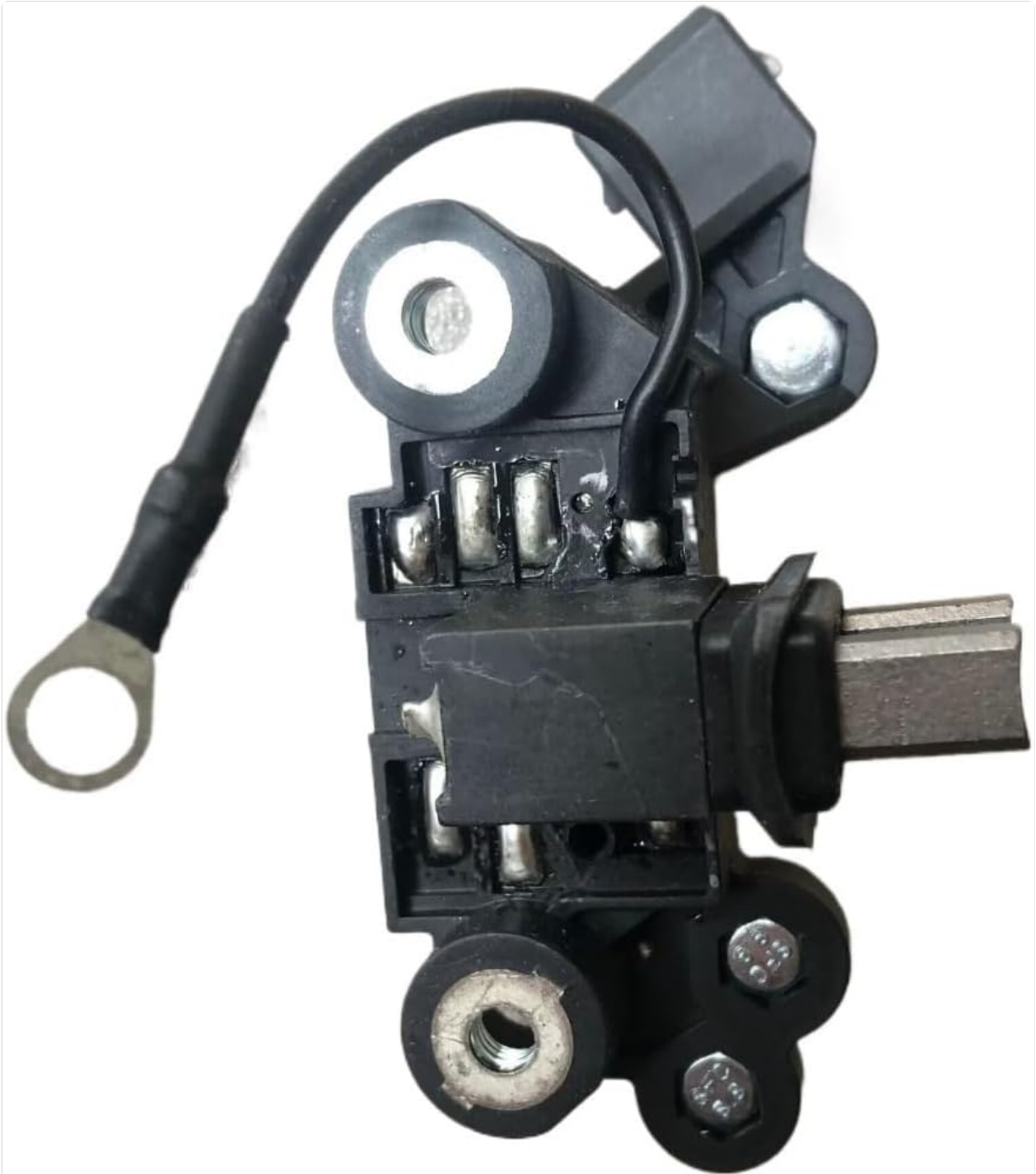
Figure 3: Angled view of the voltage regulator brush set, illustrating the brush contacts that engage with the alternator's slip rings.
