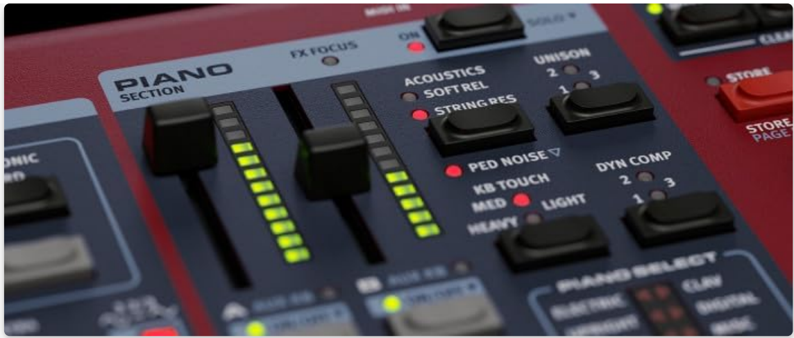
Image: Detailed view of the Piano section controls, showing faders for acoustics, soft release, string resonance, and dynamic compression.
