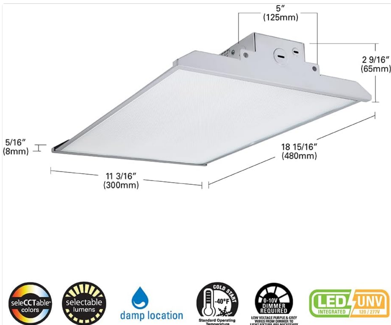
Figure 4: Detailed dimensions of the Metalux LHBS-1218C3R LED Linear High Bay Light.
