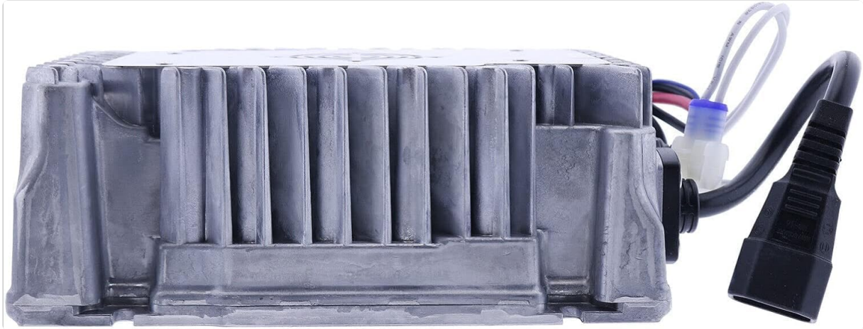
Figure 3: Side view of the charger, illustrating the various input and output ports for power and battery connections. The robust heat sink design is also visible.
