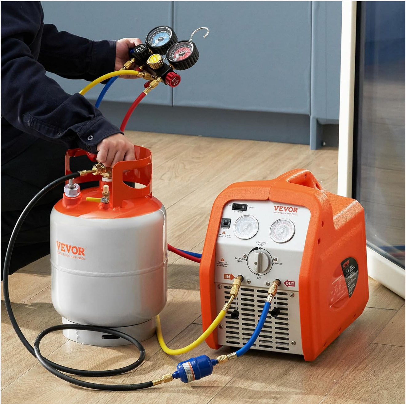
Image: A user connecting the VEVOR Refrigerant Recovery Tank to a recovery machine, illustrating the typical setup for refrigerant transfer.
