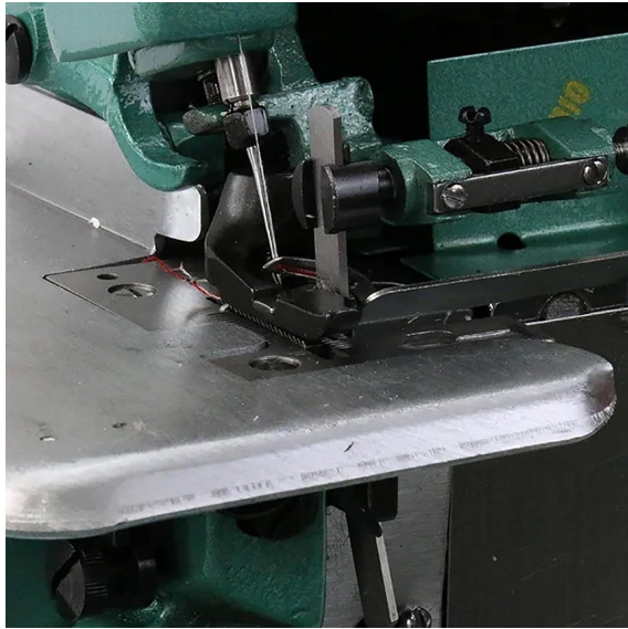
Figure 3.3: Close-up view of the needle, presser foot, and feed dogs. This detailed shot shows the critical components involved in stitching and fabric movement.
