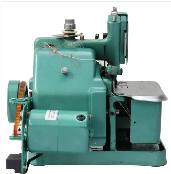
Figure 3.2: Side view of the CYMYYDS Overlocker Sewing Machine. This perspective highlights the motor housing and the belt drive system on the side of the machine.
