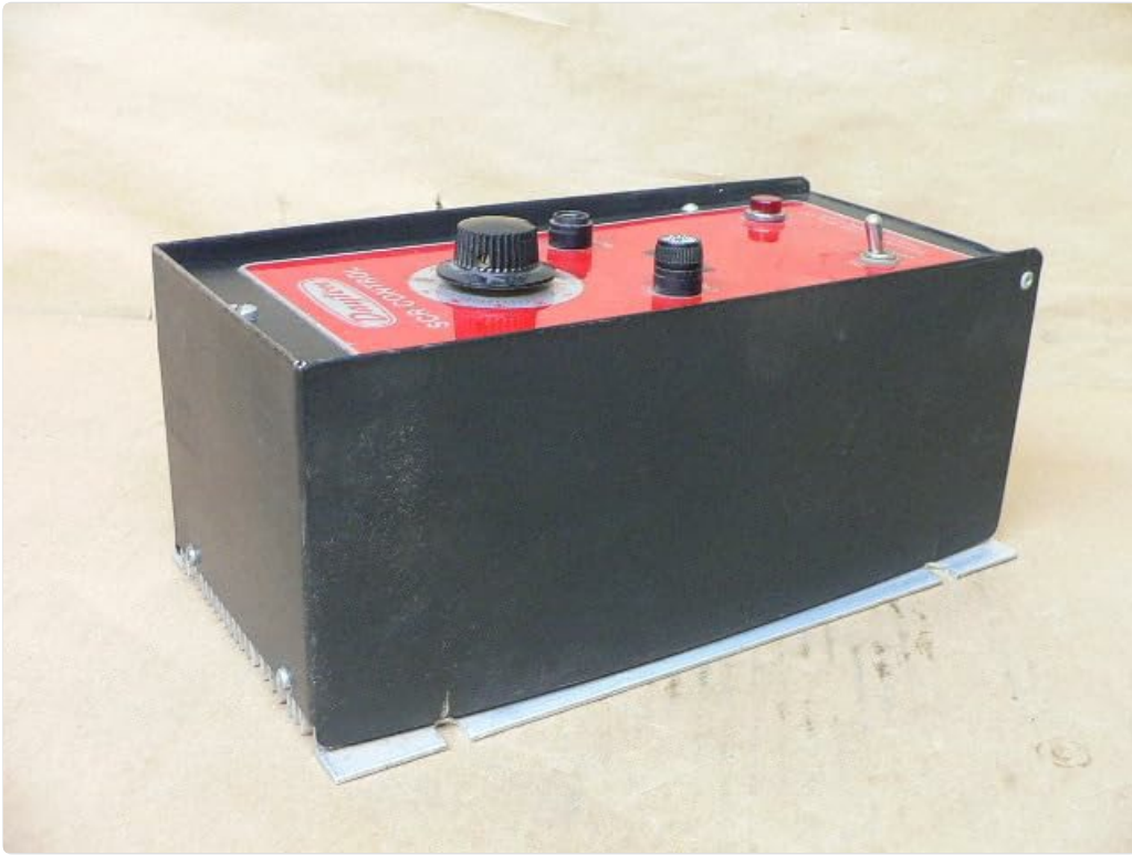
Figure 3.2: Side view of the Dayton 5X485 SCR DC Speed Control. This image highlights the overall dimensions and the metal mounting flanges on the sides of the black enclosure, indicating its design for secure installation.
