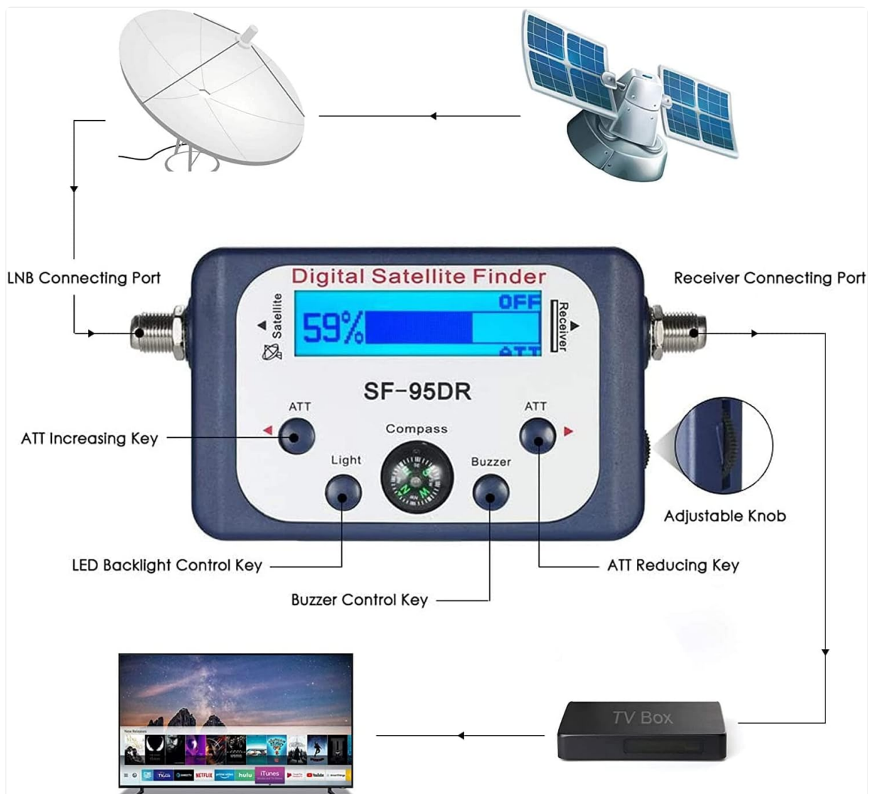
Figure 4.2: Connection diagram and labeled components of the PerGar Digital Satellite Finder SF-95DR. This diagram illustrates how the device connects between an LNB (Low Noise Block) and a TV receiver/TV box, highlighting the LNB Connecting Port, Receiver Connecting Port, ATT Increasing Key, ATT Reducing Key, LED Backlight Control Key, Buzzer Control Key, and Adjustable Knob.
