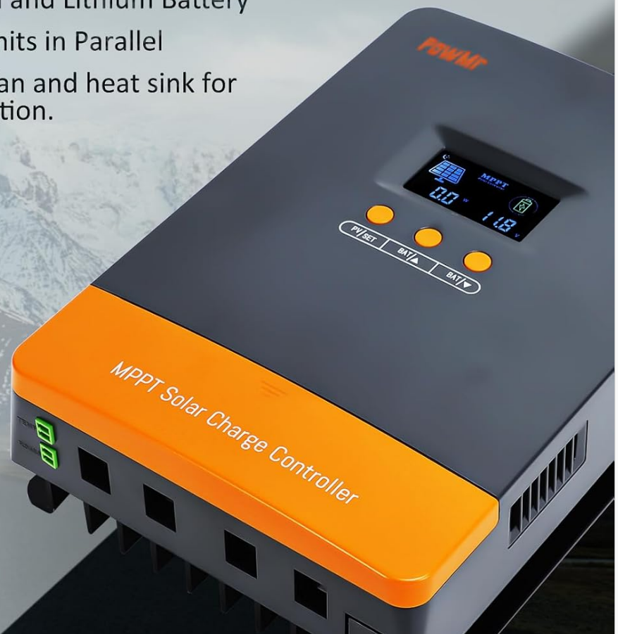
Image 2.2: Overview of the 80A MPPT Solar Charge Controller, detailing its 80A charging current, 160V maximum PV input voltage, 3840W maximum PV input power, and 8A maximum DC output current.
