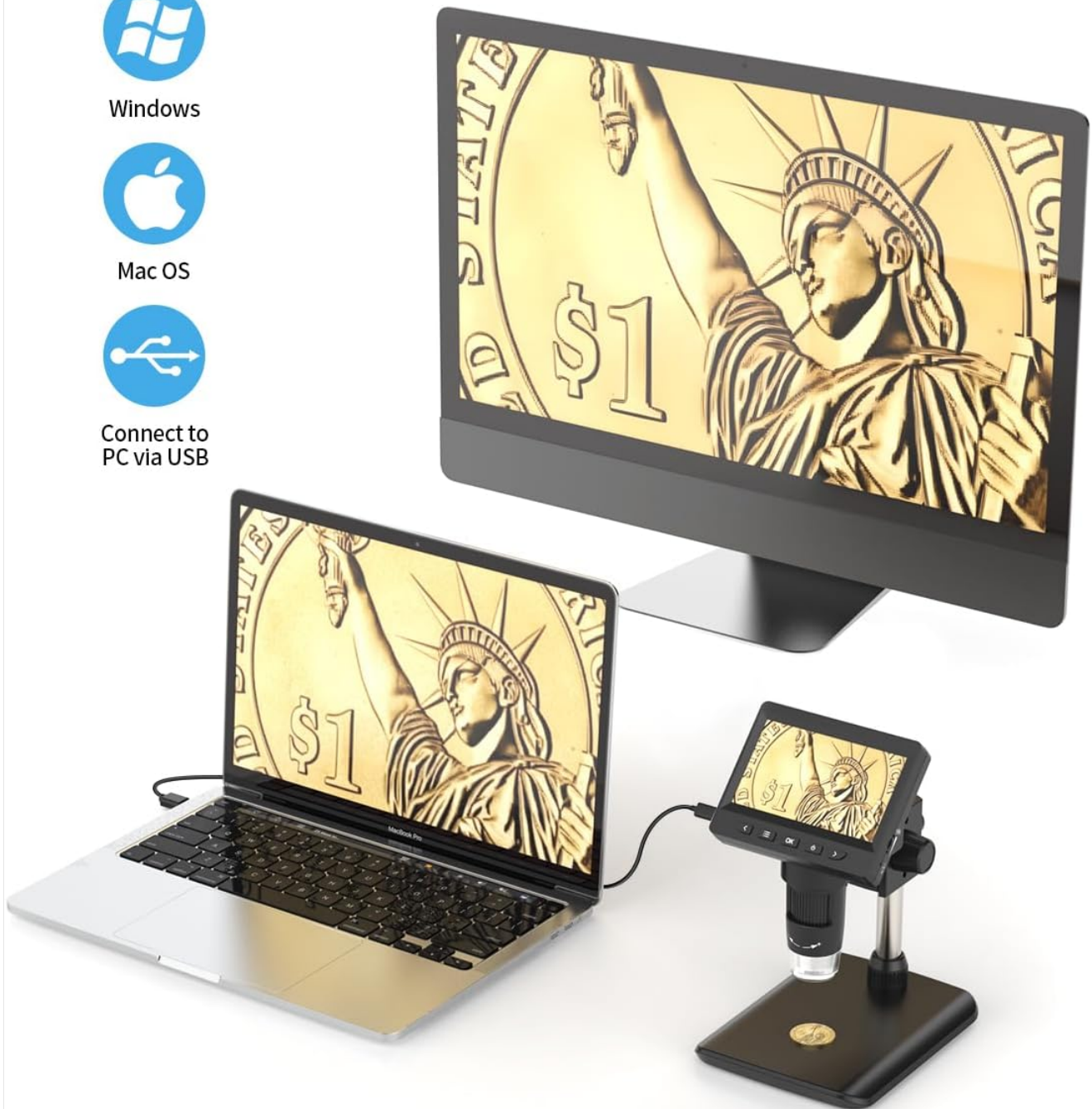
Figure 5.4: The microscope connected to both a PC monitor and a laptop, illustrating how to connect via USB for a larger image, making observation, recording, and sharing easier.
