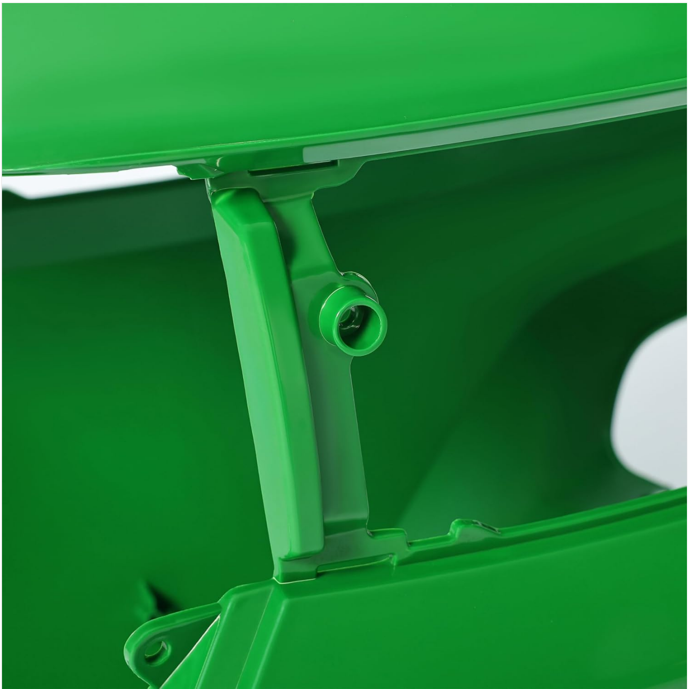
Figure 6.1: Detail of a mounting point on the HECASA Front Hood, showing where fasteners attach.
