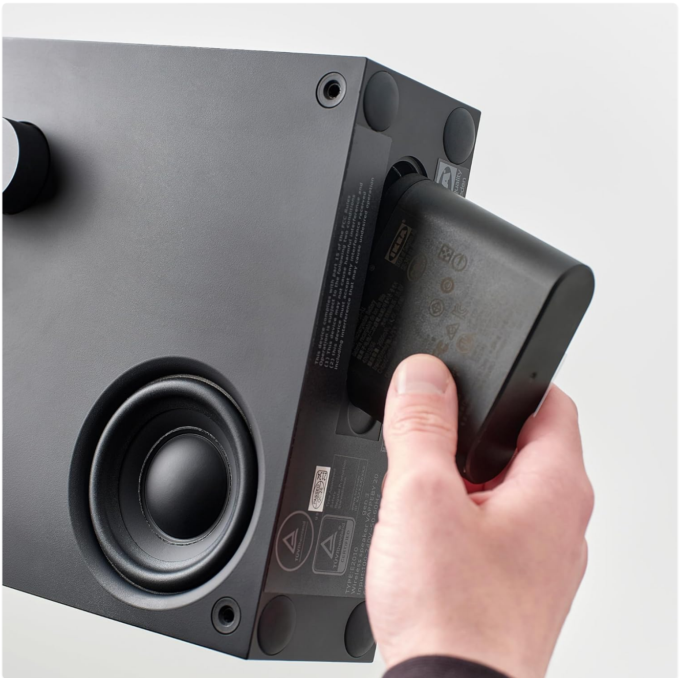
Image 3.2: Illustrates the connection point on the rear of the speaker, where the power module or battery is inserted.
