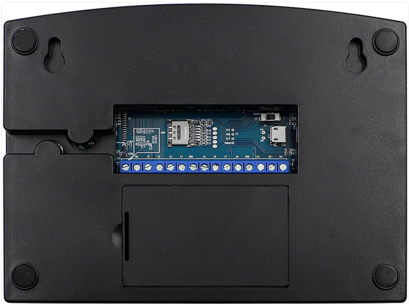
Figure 5.2: Back view of the Main Control Panel with SIM card slot and wired terminals.
