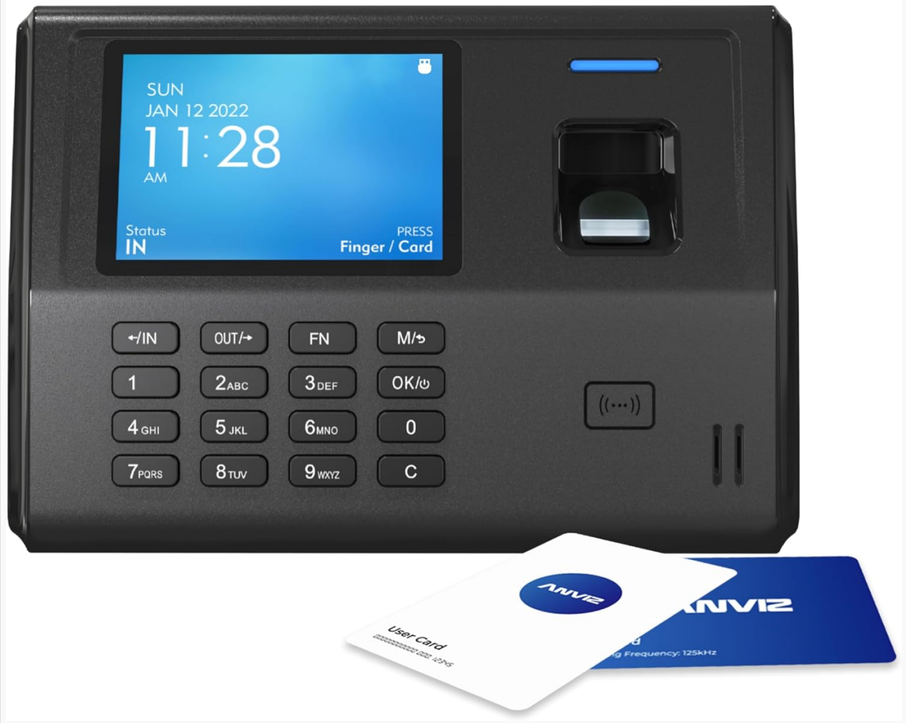
Image: The ANVIZ CX3 Time Clock with its display showing the current time and status, accompanied by two ANVIZ RFID user cards, demonstrating the card-based punching option.
