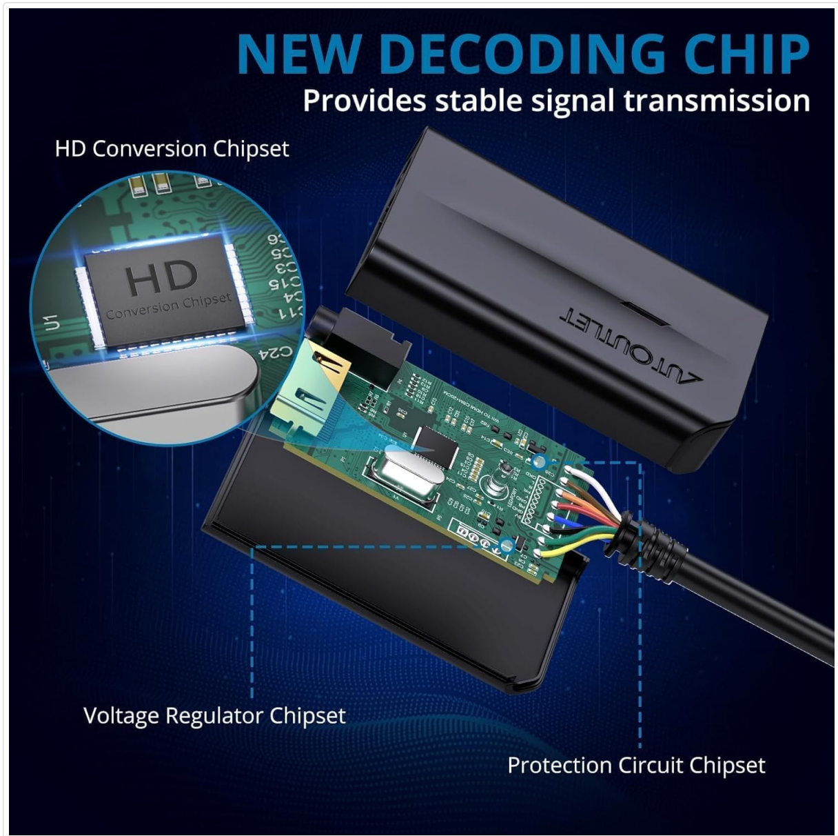
Image 3.1: Internal components of the converter, highlighting the HD Conversion Chipset for stable signal transmission.
