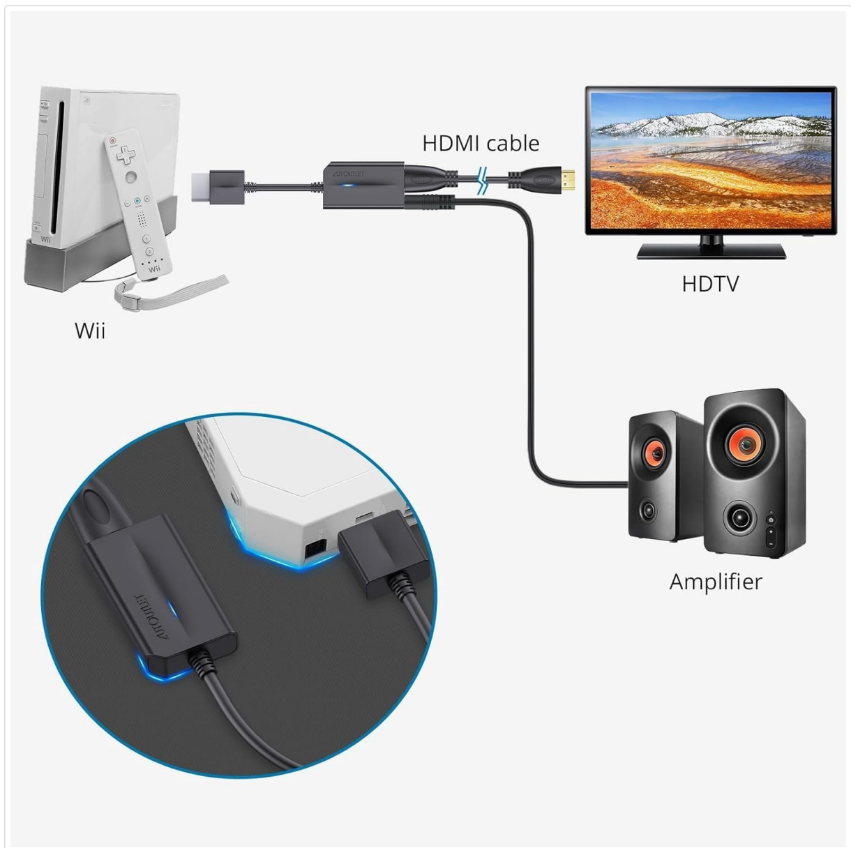
Image 4.1: Connection diagram illustrating how to set up the converter with your Wii, TV, and optional audio system.
